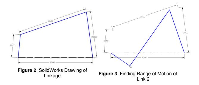
The allowable motion of the linkage can be explored by simply clicking on and dragging one of the links or joints, as shown in Figure 3. Students can easily determine that link 2 is a crank, with a full 360 degrees of motion, while link 4 is a rocker, oscillating between two limiting positions.
