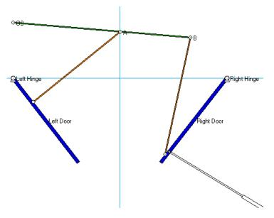
Figure 9 Barn Door Mechanism Example
