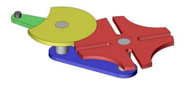
Figure 8 Geneva Wheel Mechanism Model
