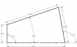
Figure 4 Finding Limiting Position of Link 4
