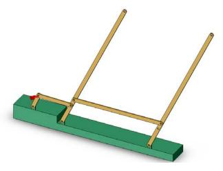
Figure 7 Wiper Assembly Model
