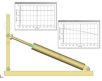
Figure 11 COSMOS/Motion Model of Cylinder Mechanism
