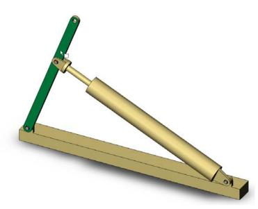
Figure 6 3-D CAD Model of Cylinder Mechanism
